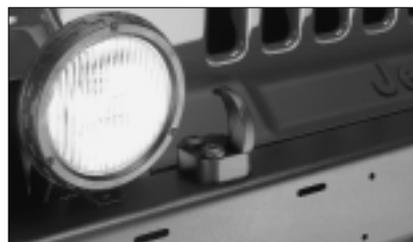
Tow Hooks mounted on OE bumper (shown on Wrangler)
