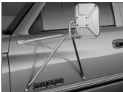
Trailer Towing Mirror, PN 82401002 (shown on Ram Pickup)
