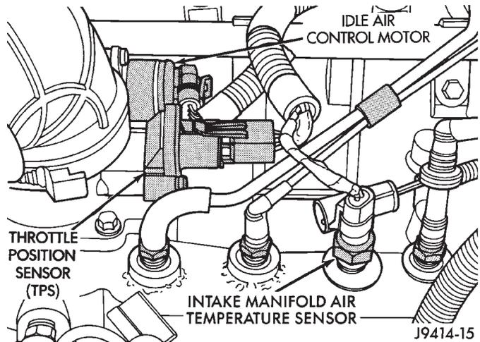
**Fig. 19 Air Temperature Sensor—4.0L Engine**
