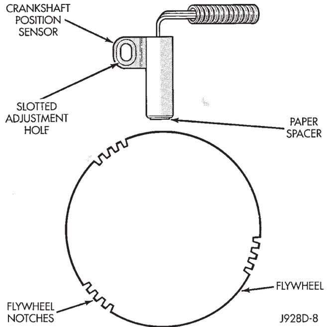
**Fig. 10 Sensor Operation—4.0L Engine—YJ Models With Automatic Transmission**
