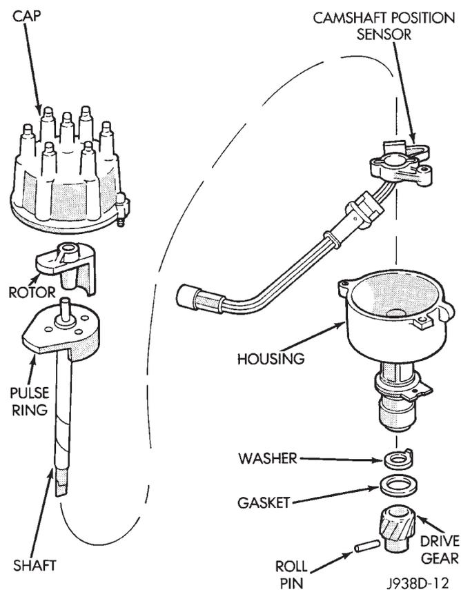
**Fig. 9 Distributor—2.5L/4.0L Engines—Typical**
