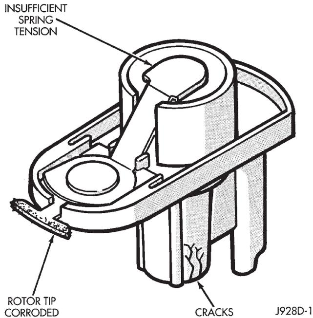
Fig. 10 Rotor Inspection—Typical
