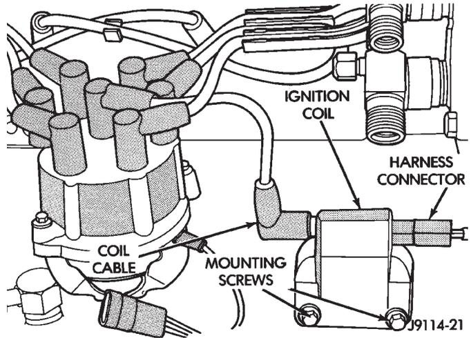
Fig. 11 Ignition Coil—Typical
