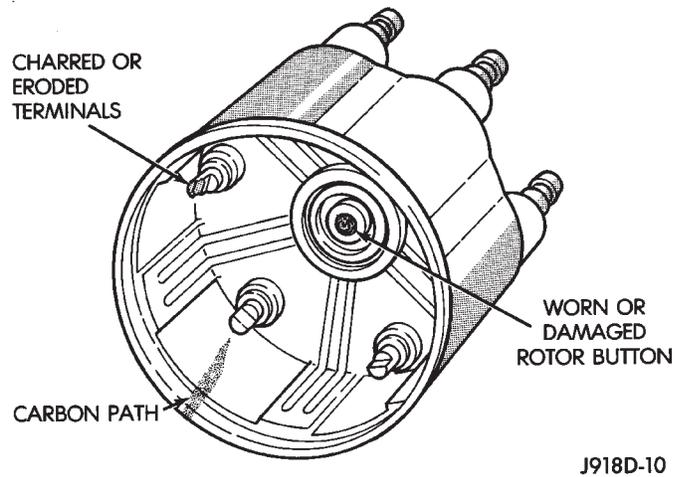
**Fig. 7 Cap Inspection—Internal—Typical**
