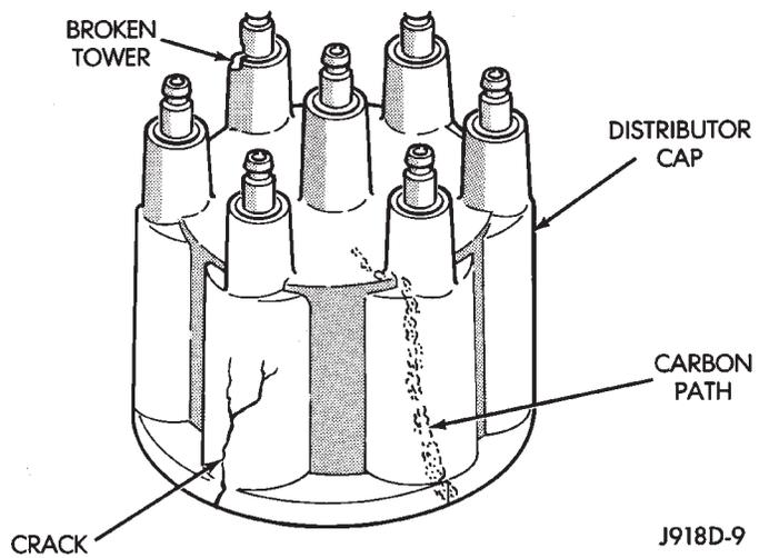
**Fig. 6 Cap Inspection—External—Typical**
